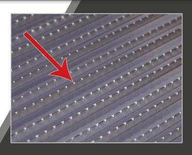
Liftgate platforms are commonly ridged side-to-side to provide traction.
